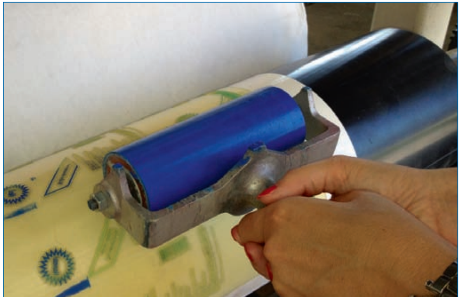
The operator can manually ink the plates and produce a proof
